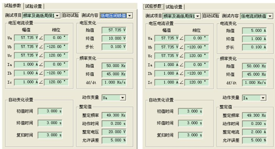
(a) 低电压闭锁值测试
